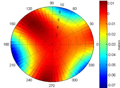
SH calibration pattern for PFM satellite antenna, E5A
